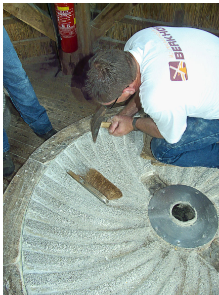
This upper burr stone turned on the lower stone to grind and pulverize wheat, which then was forced through the channels outward to be collected (Wikimedia).
